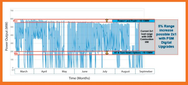
Example CCGT Plant, by combining FlexSuite and AutoTune optimization a 5% increase in load range is possible, using OEM combustor and no other hardware changes.
