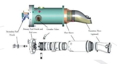
Three key design features in the LEC-III™ combustion system enable this improved process and fundamentally differentiate the LEC-III™ from the OEM design: the forward flowing venturi, effusion cooling technology, and an advanced secondary fuel nozzle (SFN).
